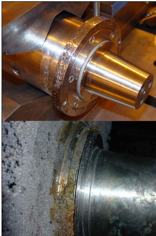
After 3 years in a grinding application at Peerless (bottom), this AirShield spindle seal continues to operate without failure.
