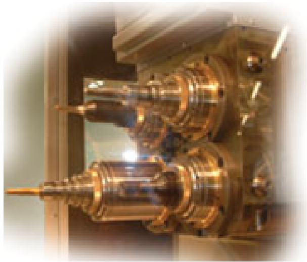
Linear toolchanger from Licon is designed for high-speed tool change in volume production.
