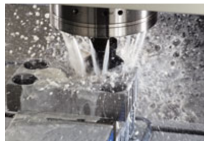
Collar above the spindle on this Hurco installation directs coolant to the work area.
