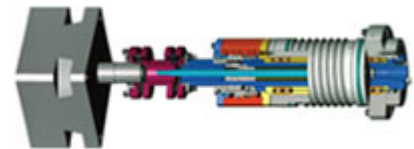
Hurco spindle uses direct drive motors.
